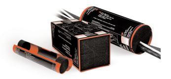
years of dependable through-penetration firestopping with no reapplication of additional product to maintain its rating. The 3M<sup>™</sup> Fire Barrier Pass-Through Device achieved up to 4 hour fire ratings (dependent upon system application) when tested by Underwriter Laboratories Inc. in accordance with ASTM E814 (UL1479).
