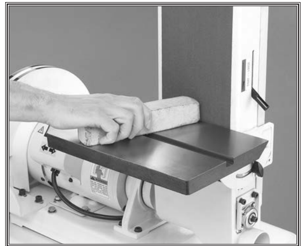
Figure 22. Cleaning the sanding belt with PRO STICK®.
