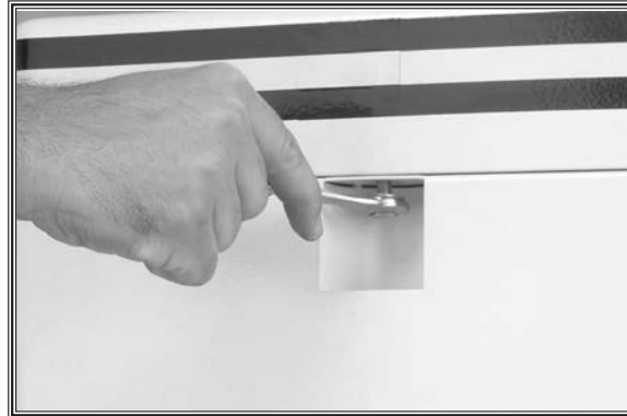
Figure 6. Mounting the sander.
