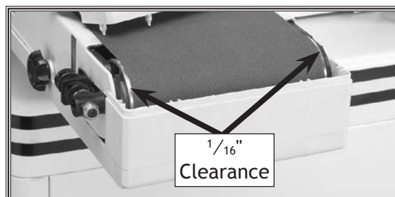
Figure 25. Proper belt tracking (guard removed for clarity).
