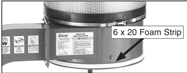
Figure 34. Example of 6 x 20 foam strip installed.
