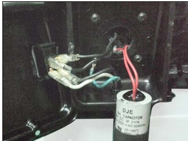
Figure 71. G0548ZP junction box, switch and run capacitor.
