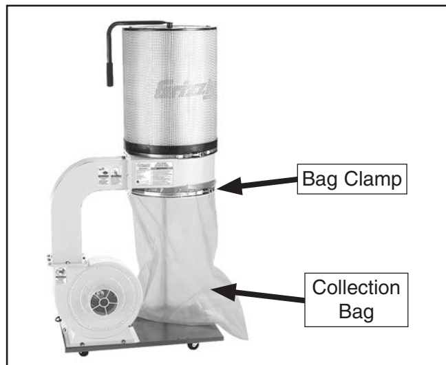
Figure 21. Collection bag installed.
