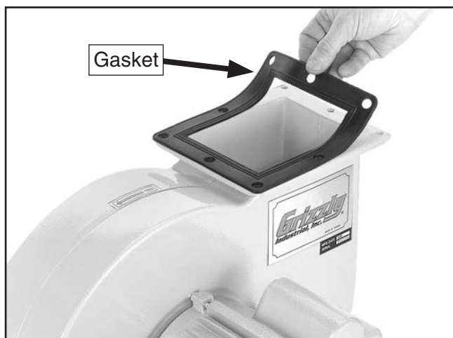
Figure 13. Positioning impeller outlet gasket.
