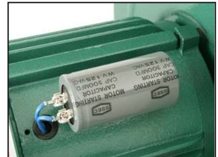
Figure 74. G1029Z2 start capacitor.
