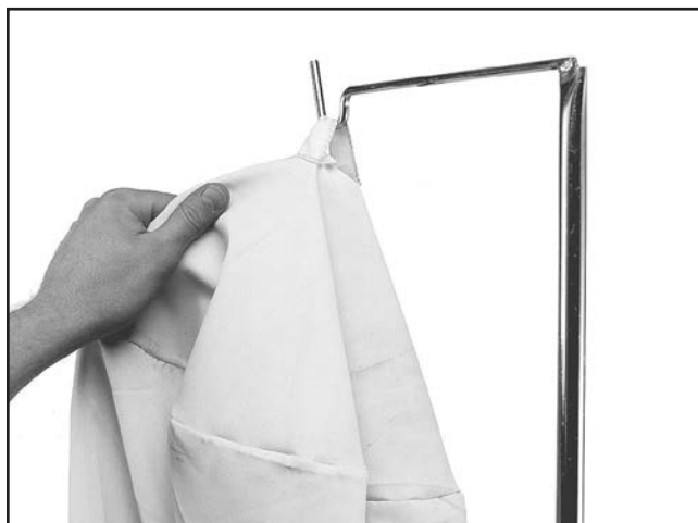
Figure 32. Attaching upper filter bag.
