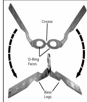
**Roof Anchor Installation:** Roof anchors must be installed in accordance with the previously discussed *Site Planning*. Site work rules, regarding when an installed Roof Anchor is ready for use (i.e. after sheathing is in place), must be followed. Figure 7 illustrates proper installation of the Roof Anchor. Install each Roof Anchor as follows:
