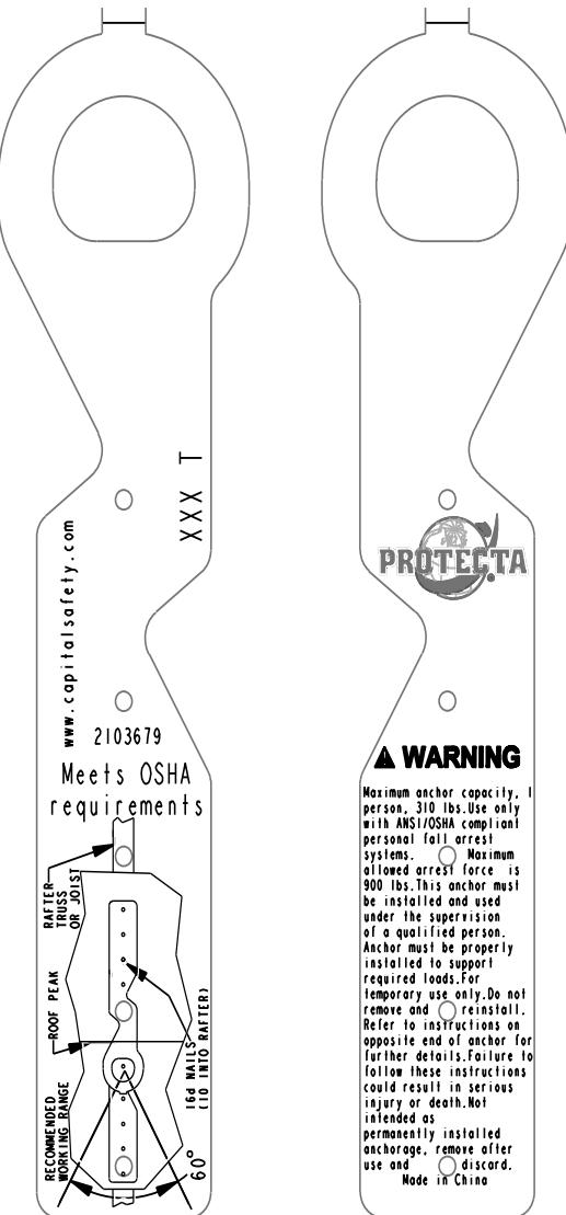
**IMPORTANT:** Markings should be legibly stamped into the Roof Anchor Base Legs.
