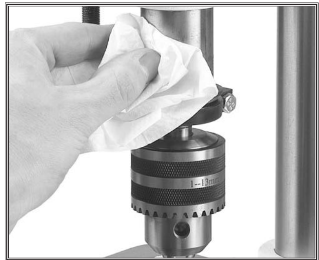
Figure 32. Clean and oil quill shaft.
