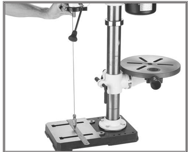
Figure 17. Aligning headstock with base.
