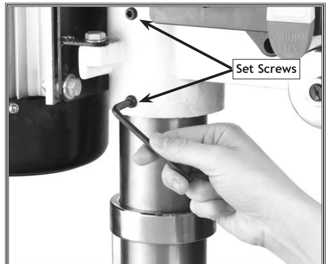
Figure 18. Securing the headstock to the column.
