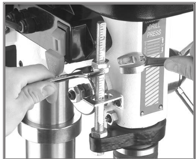
Figure 49. Back-off the depth stop nuts.
