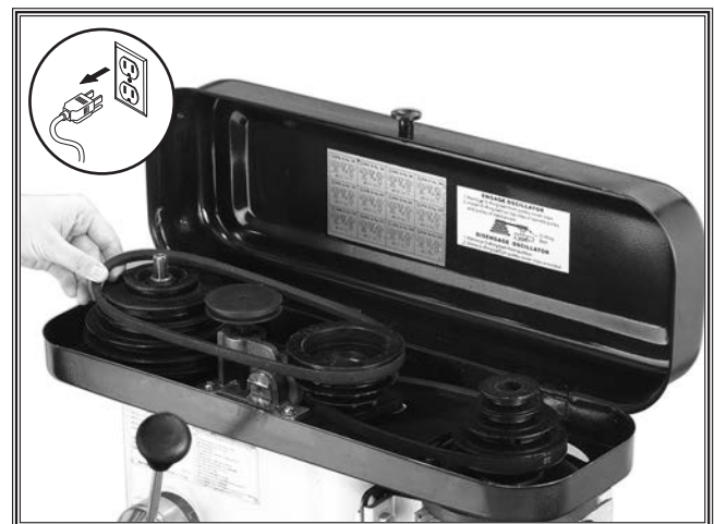
Figure 38. Adjusting belt to desired speed.
