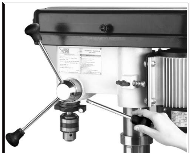
Figure 21. Installing spindle handles.
