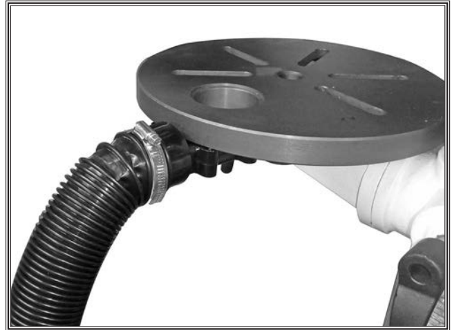
Figure 24. Dust port connected to dust collection system.
