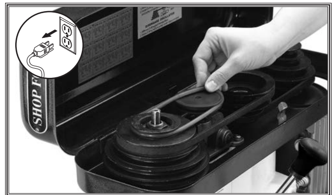
Figure 48. Stretch the belt to fit on pulleys.
