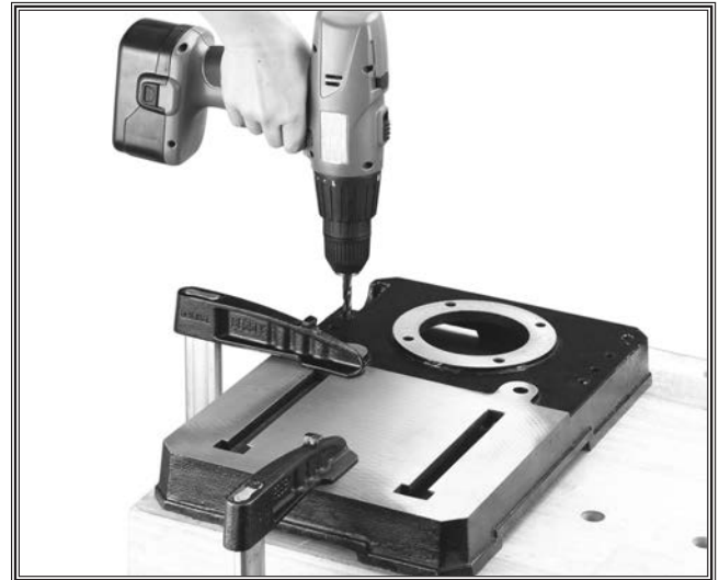
Figure 8. Using holes as a drill guide.
