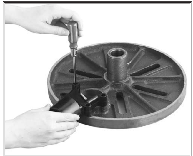
Figure 9. Installing the dust port.
