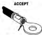
ACCEPT Wire Flush Or Greater Up To 1/32" (.032")
