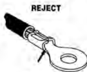
REJECT Wire Not Flush
